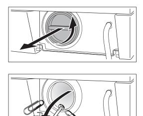
**7.** Remove any objects from the pump impeller by rotating it.
