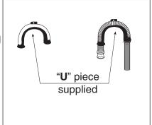
Place the drain hose into your standpipe, which should have an internal diameter of approximately 38mm thus ensuring there is an air break between the drain hose and standpipe.
